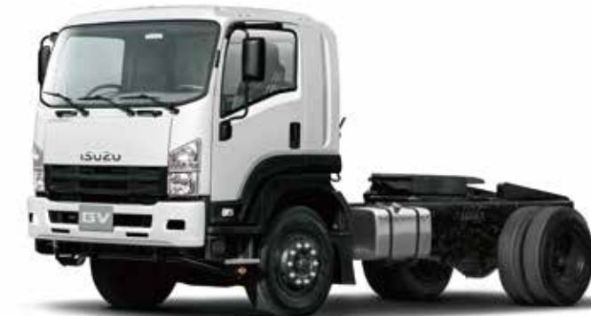
4x2 DRIVING SYSTEM ► GVR GVM 15.0ton GCM 32.0ton 6HK1-TCS
