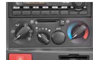
Air conditioning switch
