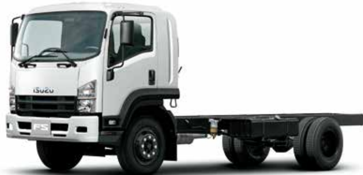
4x2 DRIVING SYSTEM ► FSR GVM 11.0ton/13.0ton 4HK1-TCS, 6HK1-TCN, 6HH1-S
